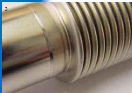
1 Automated bond welding of a 5-cornered knob 2 Bond welding of a stainless steel profile, material thickness 0.8 mm 3 Bond welding of a tube to an expansion joint, stainless-steel components with material thickness 0.1 mm
